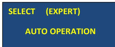
On this screen, pressing “ENT” key would put the unit in Auto Operation. This mode would continue till alternate option mode is selected or unit is put in Power down condition.
