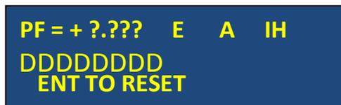
Pressing the Enter key, would reset the **VH / IH** fault even if voltage / current THD% is above the set limit. The fault indication would continue till the respective THD% is above the set limit. In case of THD% above limit, all capacitor banks are switched off to protect them.
